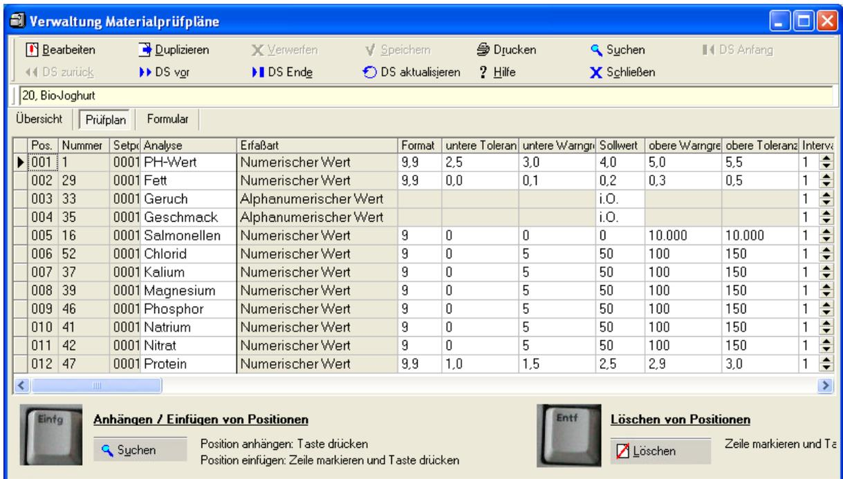
The screenshot shows the 'Verwaltung Materialprüfpläne' window with a menu bar and a table of analysis parameters. The table has columns for Pos., Nummer, Setp, Analyse, Erfasart, Format, untere Toleranz, untere Warngre, Sollwert, obere Warngre, obere Toleranz, and Interv.
